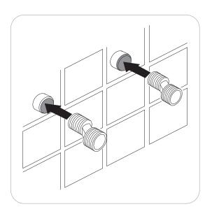
1. Screw in offset connectors (18) to water feed sections ending with female thread G1/2, sealing the connection with an appropriate amount of teflon tape or thread. After the installation, the axes of openings in the offset connectors (from the tap side) must be at the same height, their face surfaces at the same distance from the wall, and the spacing of the openings equal to the distance between axes of connection nuts of the tap body.
